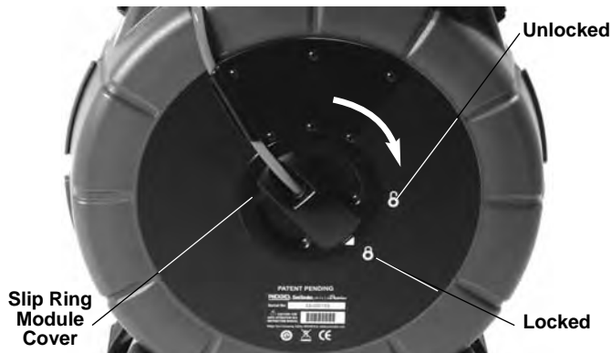
Figure 11 – Locking The Slip Ring Module Cover
