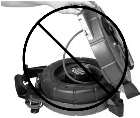
Figure 10 – Do Not Allow Cable to Uncoil Freely
