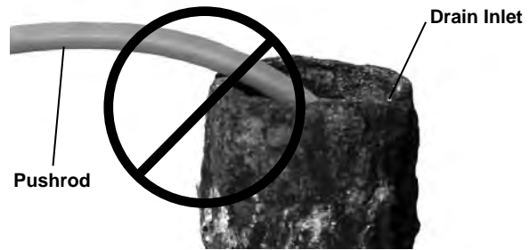
Figure 23 – Avoid Pulling At Sharp Angles
