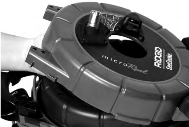
Figure 5 – Open Drum Carefully To Route Cable
