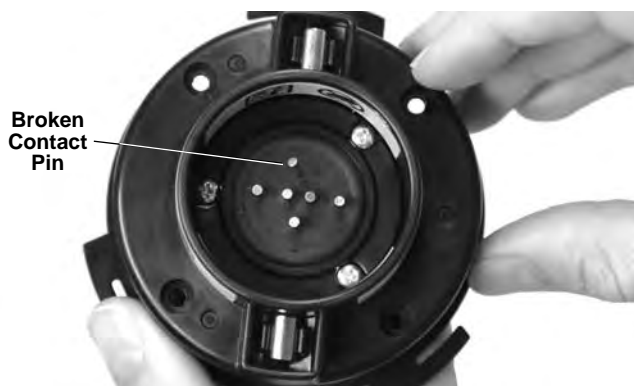
Figure 12 – Broken Contact Pin
