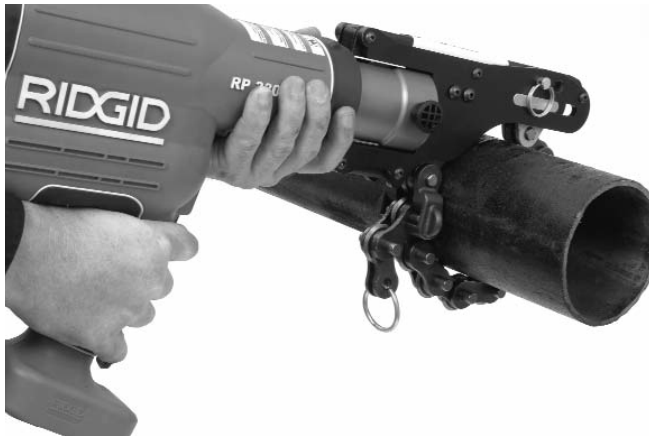
Figure 5 – Cutting The Pipe
