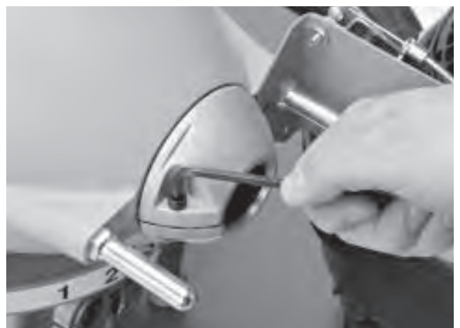
Figure 13 – Removing Clutch End Play
