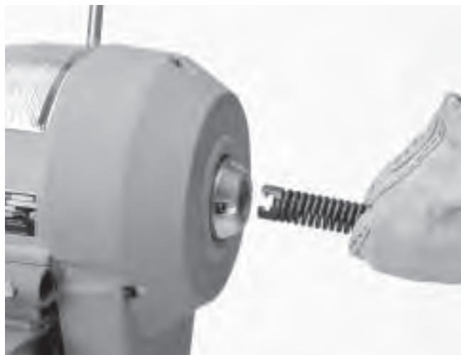
Figure 3 – Inserting Cable Into Front Of Machine
