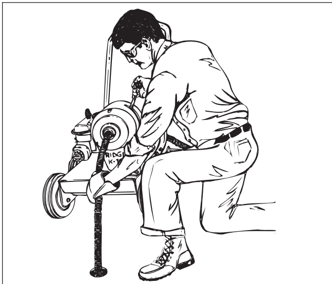
Figure 5 – Operating Drain Cleaning Machine
