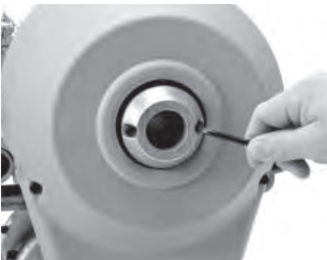
Figure 11 – Replacing Clutch Jaws
