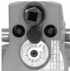
Figure 5 – Gauge In Grooving Position
