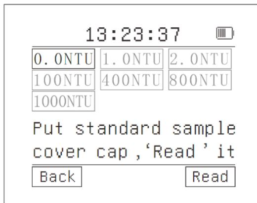
3. Click "Back" to cancel the calibration and return to the main interface. Click "Read" to enter the "Checking" interface. Automatically switch to the next calibration point, and then complete the calibration of 4 calibration points of 0/1/2/100 NTU.
