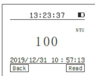
5. After the test result is displayed, click "Back" to return to the main interface; click "Read" to perform the next test.
