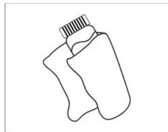
1. Add more than 10ml of the solution to be tested, tighten the bottle cap, and add carefully to avoid air bubbles.
