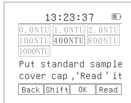
4. After completing the first 4 points calibration, the subsequent calibration interface adds "switch" and "complete" two functions.
