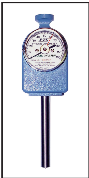
Model 307LCRBIV Durometer for measuring shell hardness of Dungeness crabs
