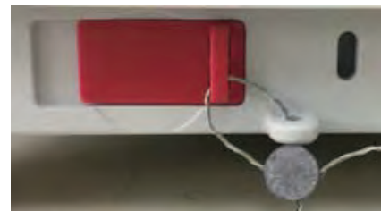
Locked with Wire Seal
