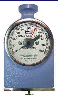
The Model 302SL Foam & Rubber Durometer is a unique instrument that measures the hardness of soft materials such as foam rubber, sponge rubber, cellular material and gel-like materials.
