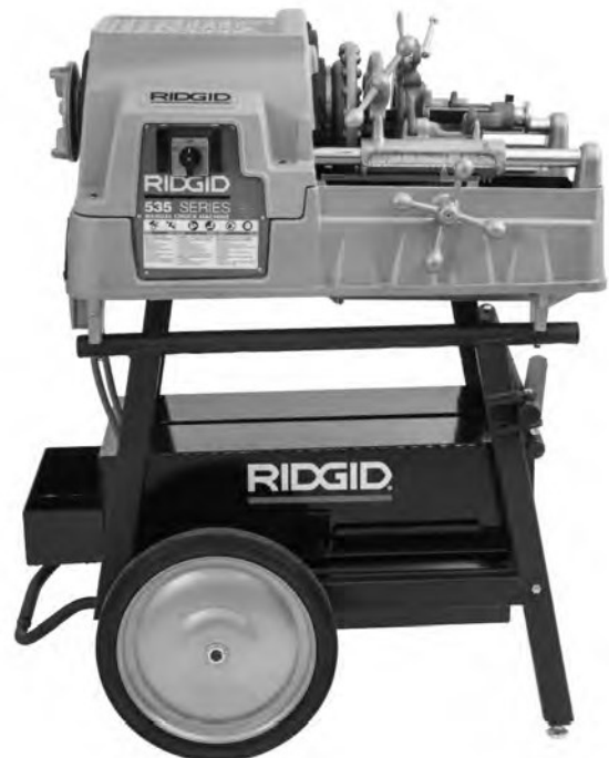
Figure 28 – Machine prepared for Transport
