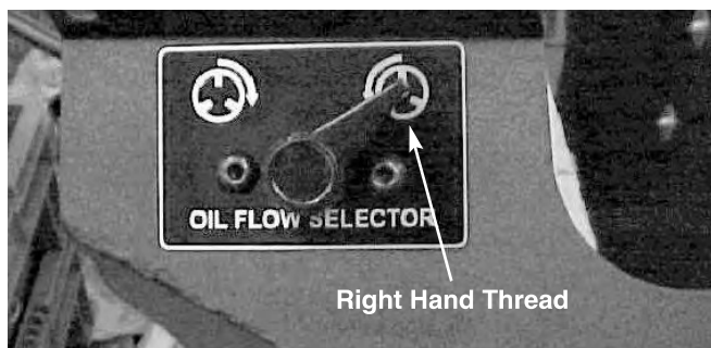
Figure 24 – LH or RH Oil Flow Selector
