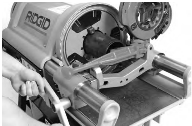
Figure 22 – Reaming Pipe with Reamer
