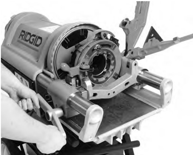
Figure 23 – Threading Pipe (714 Die Head Shown)
