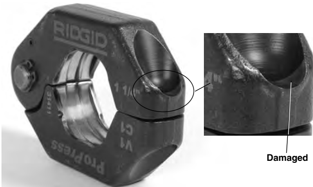
Figure 13 – Damaged Ring Pocket
