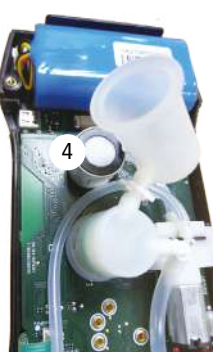
New sensor connected to electronic board
