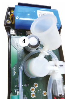
New sensor connected to electronic board
