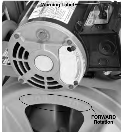
Figure 8 – Proper Drum Rotation (FOR Switch Position)
