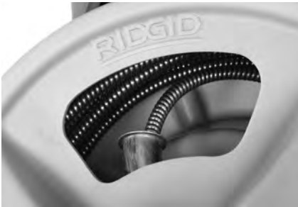
Figure 18 – Coil Cable Into Drum As Shown
