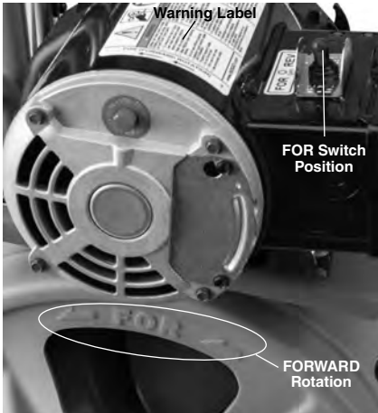
Figure 8 – Proper Drum Rotation (FOR Switch Position)
