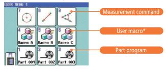
\* A user macro is a measurement command created by the user, and is a combination of several standard **QM-Data200** measurement commands. Note: Up to three user menus, from [USER1] to [USER3], can be registered. A maximum of nine icons can be registered for one menu.
