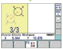
Next, the measurement navigation procedure for round hole B will be displayed. Determine each position (b1, b2, b3) in the same manner as in step (2).
