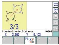
Determine each position (a1, a2, a3) on round hole A, following the measurement navigation procedure on the LCD.
