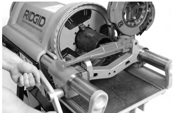
Figure 22 – Reaming Pipe with Reamer
