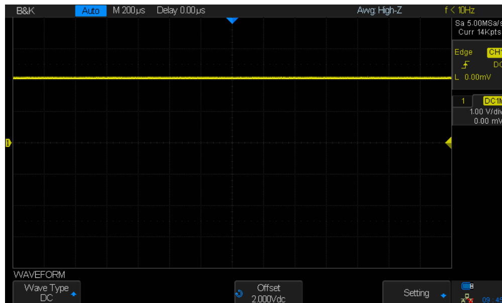
Figure 138 Default DC Waveform
