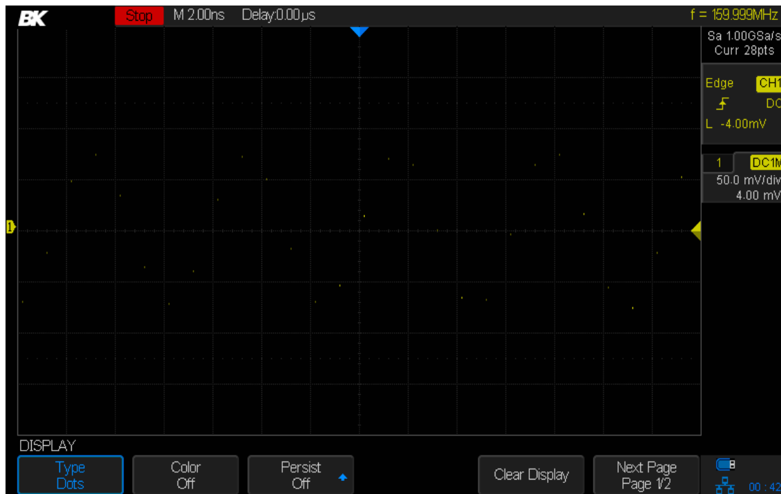
Figure 30 - Display type set to dots
