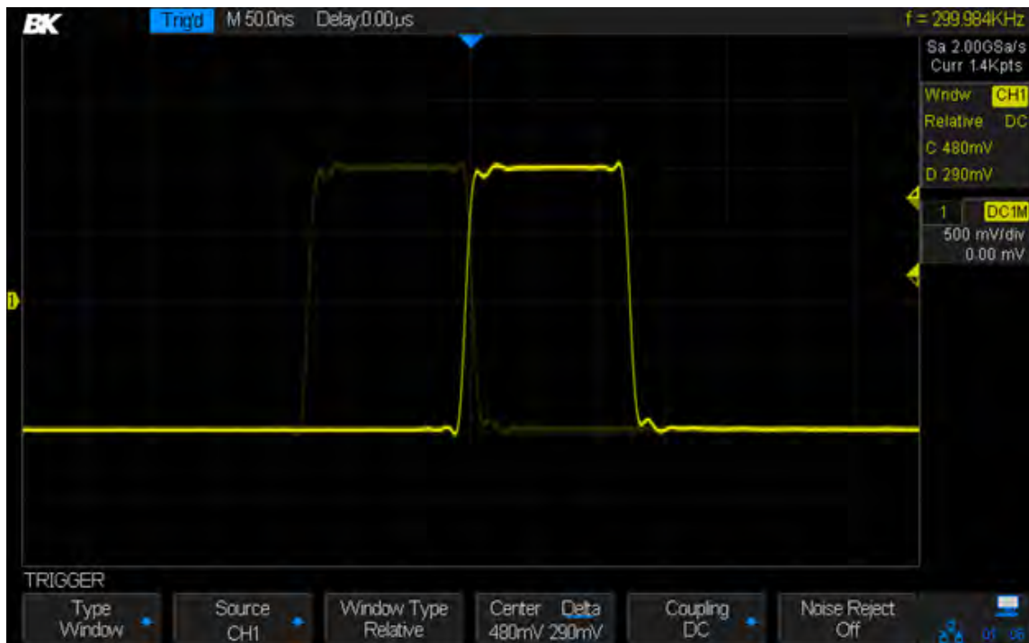
Figure 57 - Relative window trigger
