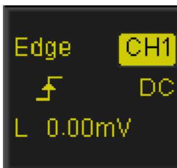
Figure 5 - Trigger settings display
