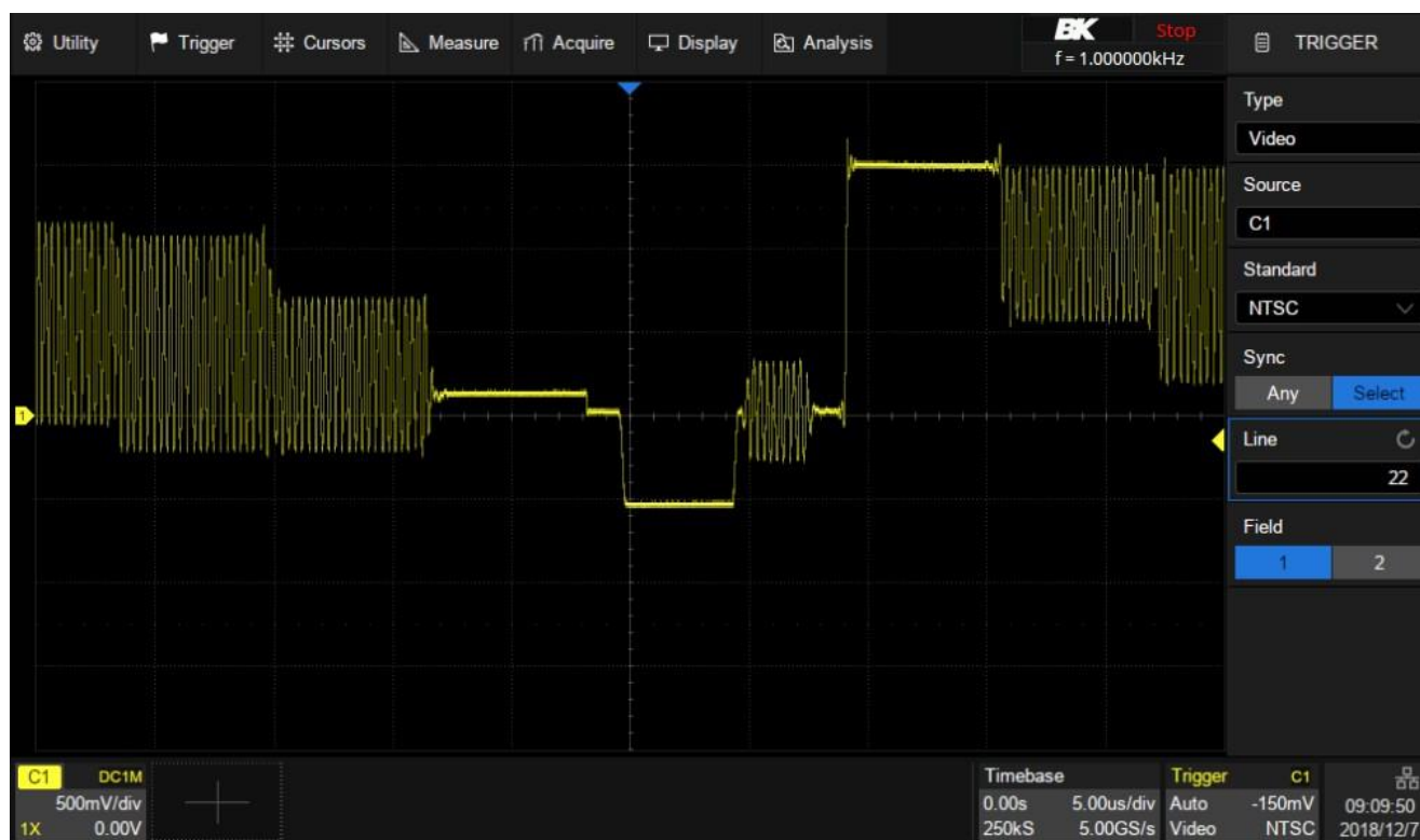
Figure 9.14 Triggering on a Specific Line of Video
