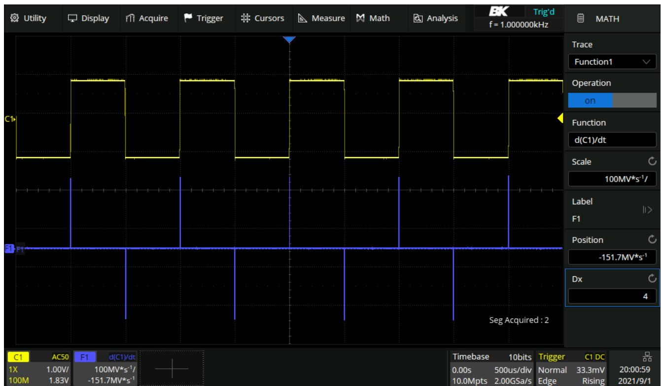
Figure 13.6 Difference Function Operation
