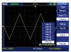
Minimize debug time by saving and recalling setups and waveforms from internal memory. Save and recall up to 20 different oscilloscope setups and 10 different waveforms.
