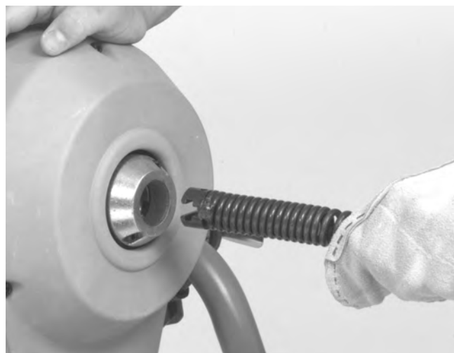
Figure 4 – Inserting Cable Into Front Of Machine
