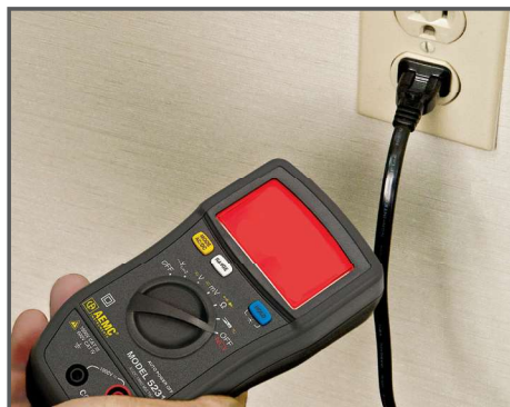
Non-contact detection of network voltage (NCV Function-AC only)
