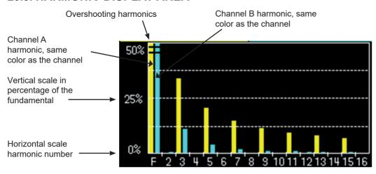
This area displays harmonics 1 to 16 of the validated channels in the form of a bar chart. The user can switch from the display of harmonics 2 to 16 to the display of harmonics 17 to 31. The max. vertical scale will depend on the zoom factor. The zoom factor can be modified using the Acq menu.
