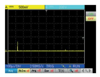
■ with PkDet (the detection of the min and max obtained between two sampling steps makes it possible to view all the combs):
