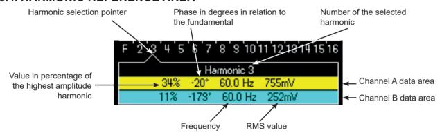
This window displays the specific measurements of the selected harmonic for each channel. The following measurements are displayed:
