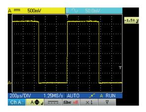
Turn the screw in either direction until the signal is horizontal and looks like the screen shown opposite. Your sensor is now calibrated, so you can turn the BNC base again to close access to the adjustment screw.
