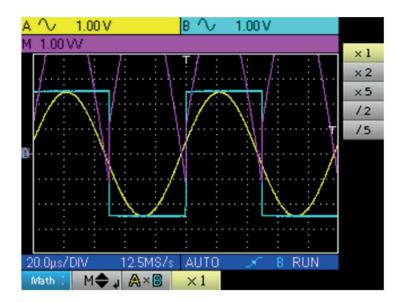
In our example, the peak amplitude of our mathematical function is 2.5 V \* 2.5 V = 6.25 VV. As the channel M sensitivity is 1 VV (with the factor x 1), it can be seen that the trace overshoots and can be corrected by using the /2 coefficient.
