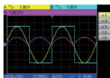
As the positive voltages of signals A and B are equal, the division leads to a positive peak voltage of 1 V/V, and therefore a representation of 1 division on the trace. This can be expanded by choosing factor x 2 or x 5:
