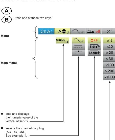
selects the channel filter (OFF, 5 kHz, 1.5 MHz)
