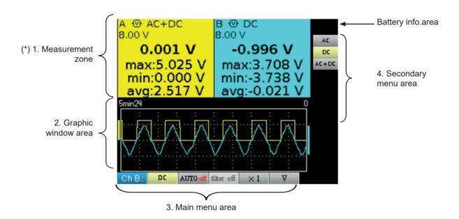
(\*) If the measurement is not possible, dotted lines will be displayed. If the channel is not validated the measurement will be replaced by "-x-".
