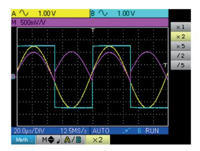
The sensitivity of channel M changes to 500 mV/V and the positive peak amplitude of the trace is 1 V/V.
