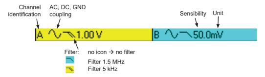
The direct data from channels A and B are displayed in this window:
