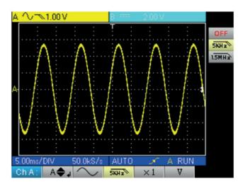
■ with the 1.5 MHz low-pass filter (the sinusoidal is partially cut):
