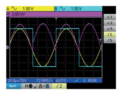
The sensitivity of channel M becomes 2 VV and the peak voltage is 3.125 \* 2 VV = 6.25 VV.
