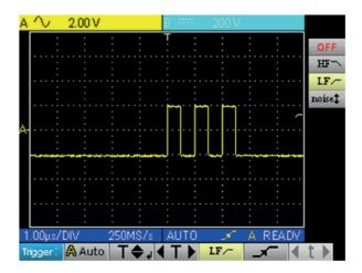
This can also be achieved without a filter, but by slecting triggering on a pulse width of less than 1 µs :
