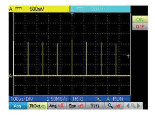
Peak detection deactivates ETS (Equivalent Time Sampling) reconstruction of a repetitive trace. Sampling is real-time for time bases ≤ 2.5 µs/div.
