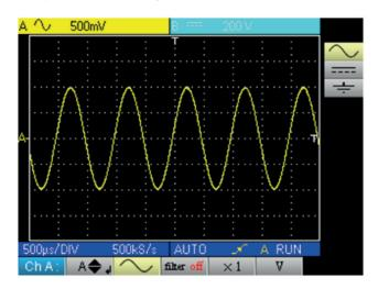
■ with DC coupling (the entire signal is measured):
