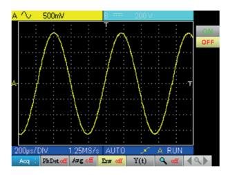
■ with envelope (an acquisition is displayed at each triggering):
