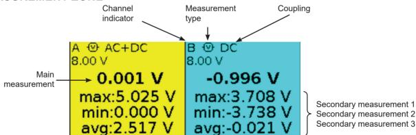
The direct data from channels A and B are displayed in this window:
