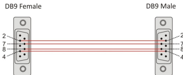
Figure 27 – Building an extension cable
