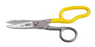
These Scissors are free-fall snips that feature stainless steel blades for blade sharpness and durability. They cut 19 AWG and 23 AWG electrical communication wire, cable and cordage. The extended handle allows for more comfortable cutting and provides leverage during wire cutting. The free-fall design makes this snip easier to use.
