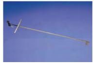
T-handle with  $\frac{3}{8}$ " penetration to check moisture in stacks in or out of kiln.
