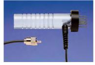
Eight insulated 1 ½" pins with 1" penetration. Used for yarn.
