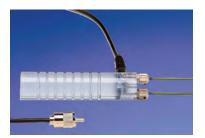
Two insulated 9 ½" pins with 8 ¼" penetration. Used for baled cotton.
