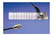
Eight pins with <sup>1</sup>/<sub>8</sub>" penetration and adjustable penetration depth. Used for veneer, leather, or paper.
