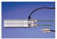
Two insulated pins with 3 1/4" penetration. Used for roofs, insulation, or EIFS.
