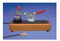
Clamp type for testing thin sheet stock, veneer, and fiberboard between two smooth disks.
