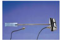
Double-roller type. Used for paper or textile on moving web.
