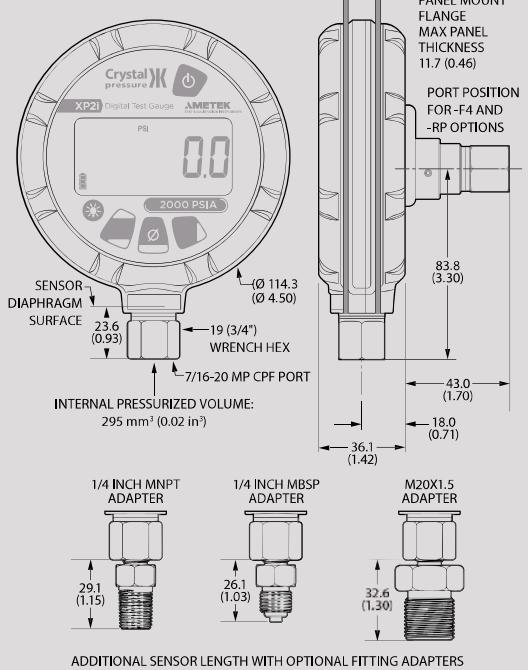
ADDITIONAL SENSOR LENGTH WITH OPTIONAL FITTING ADAPTERS
