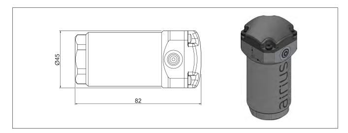
Airius is a wireless, battery-powered sensor that performs a user-defined number of vibration measurements per day in the 10-1000 Hz or the 2-1000/10-5000 Hz frequency range. The MEMS (micro-electro-mechanical-systems) type sensor with digital output measures triaxial vibration and temperature.
