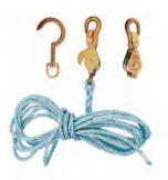
All Klein block and tackle use high-quality, 3/8-lnch (10 mm) diameter rope. Light, galvanized-steel shell blocks are fitted with snubbing hooks to hold the load. This package features two blocks with a swival Klein hook Cat. No. 259 with a maximum safe load of 750-pound (340 kg).
