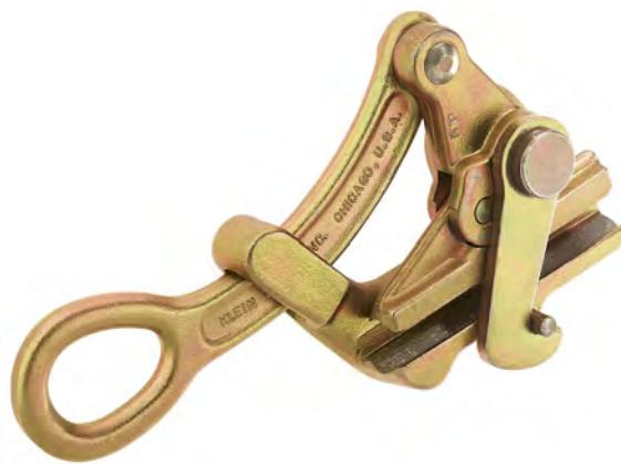
Longer knurled jaws achieve a firm hold, reducing possibility of slippage and damage to cable. Design includes a latch, plus a large-diameter eye that accommodates large hooks on hoists, winches and tackle blocks. When latch is closed, it helps maintain cable position in grip jaws.
