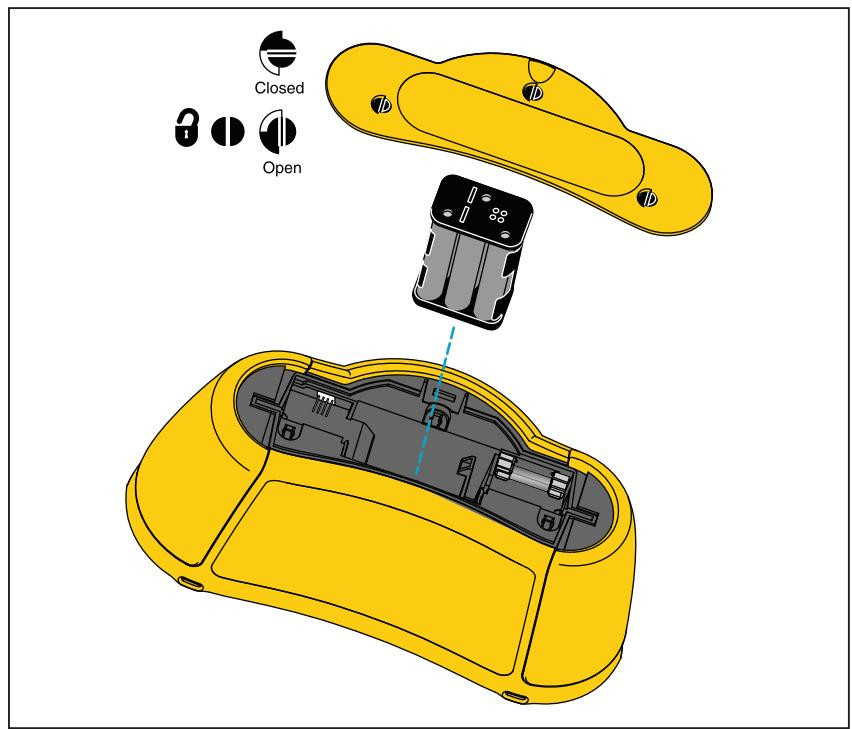
**Figure 17. Battery Replacement**
