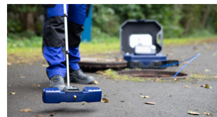
With the Wohler L 200 Locator, the camera head can be located with pinpoint accuracy.
