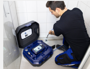
The waterproof camera head enables the inspection of sewers, among other things.
