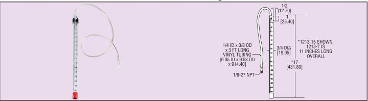
**Provide visual indication of pressure** with the Series 1213 Gas Pressure Manometer. Designed for use with natural gas, the manometer can also be used to monitor any compatible gases up to 15 inches of water column. Tap water is used as the sensing media and a magnetic clip provides temporary or permanent mounting. Economically priced and made of durable plastic for years of trouble-free service. Includes 3' of vinyl tubing and 1/8" nylon male NPT to barb fitting.
