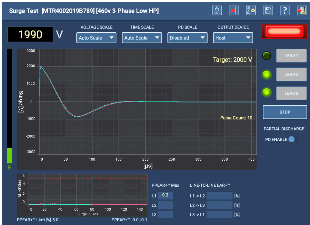
Fig 111: Auto Surge test screen—test in progress.
