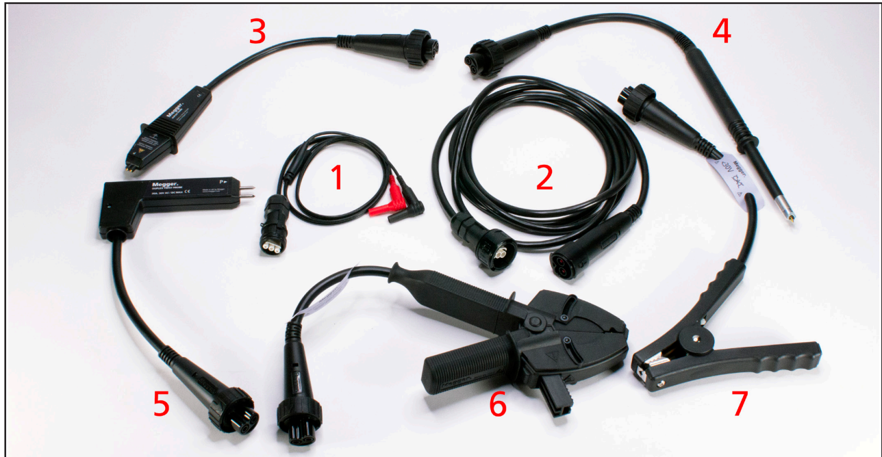
Fig 19: Megger DLRO Connect system for low-voltage testing using the RLC adapter.
