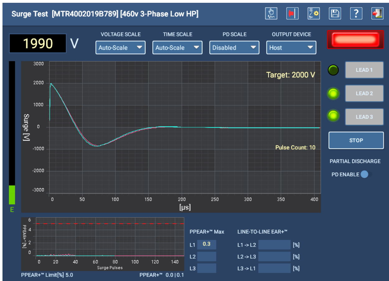
Fig 125: Auto Surge test screen.
