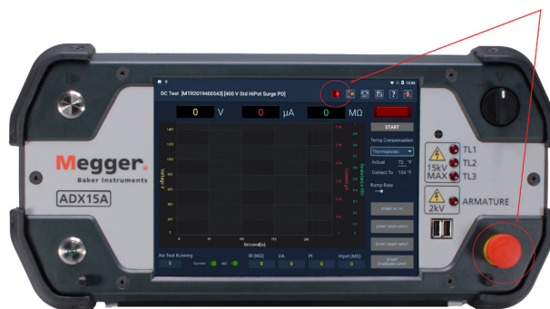
Fig 2: Megger Baker ADX showing Equipment Stop button.
