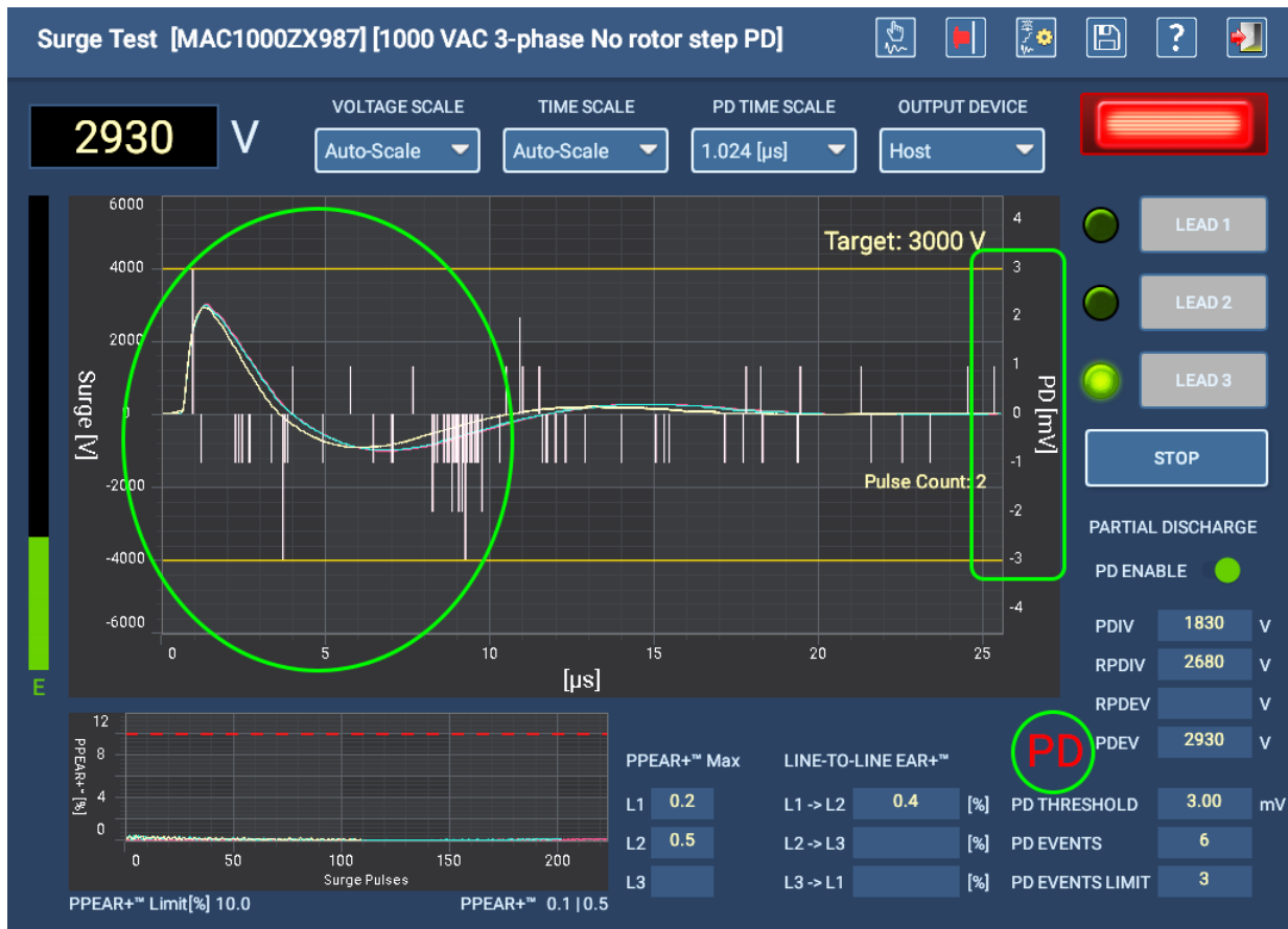
Fig 113: ADX Surge Test screen with PD enabled and values recorded.
