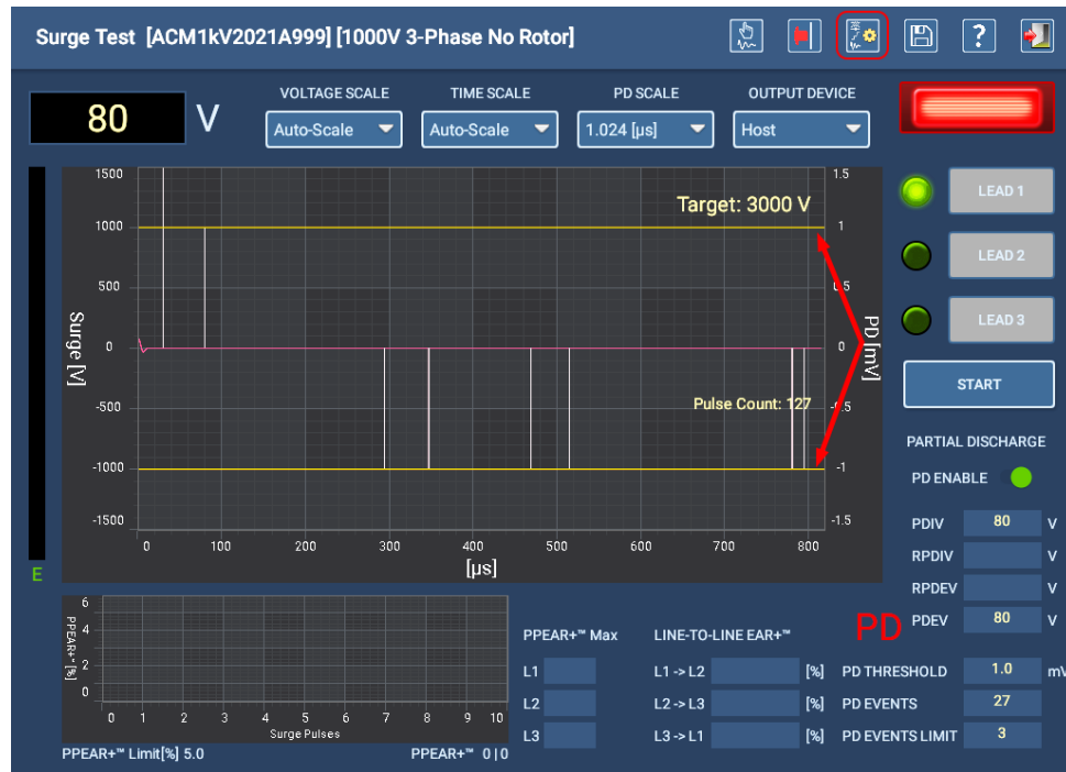
Fig 117: Surge Test screen in Manual mode for setting PD parameters.
