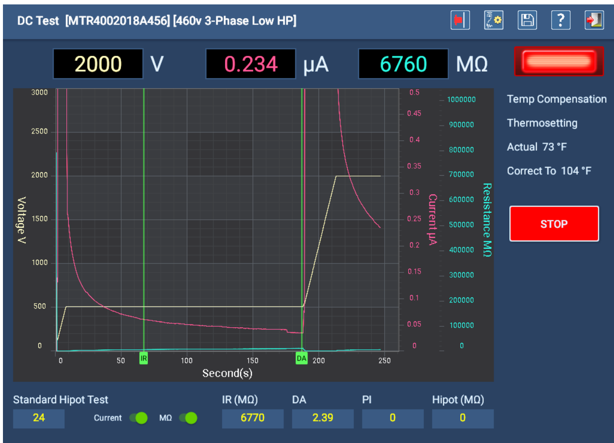
Fig 124: Auto DC Test screen—test in progress.
