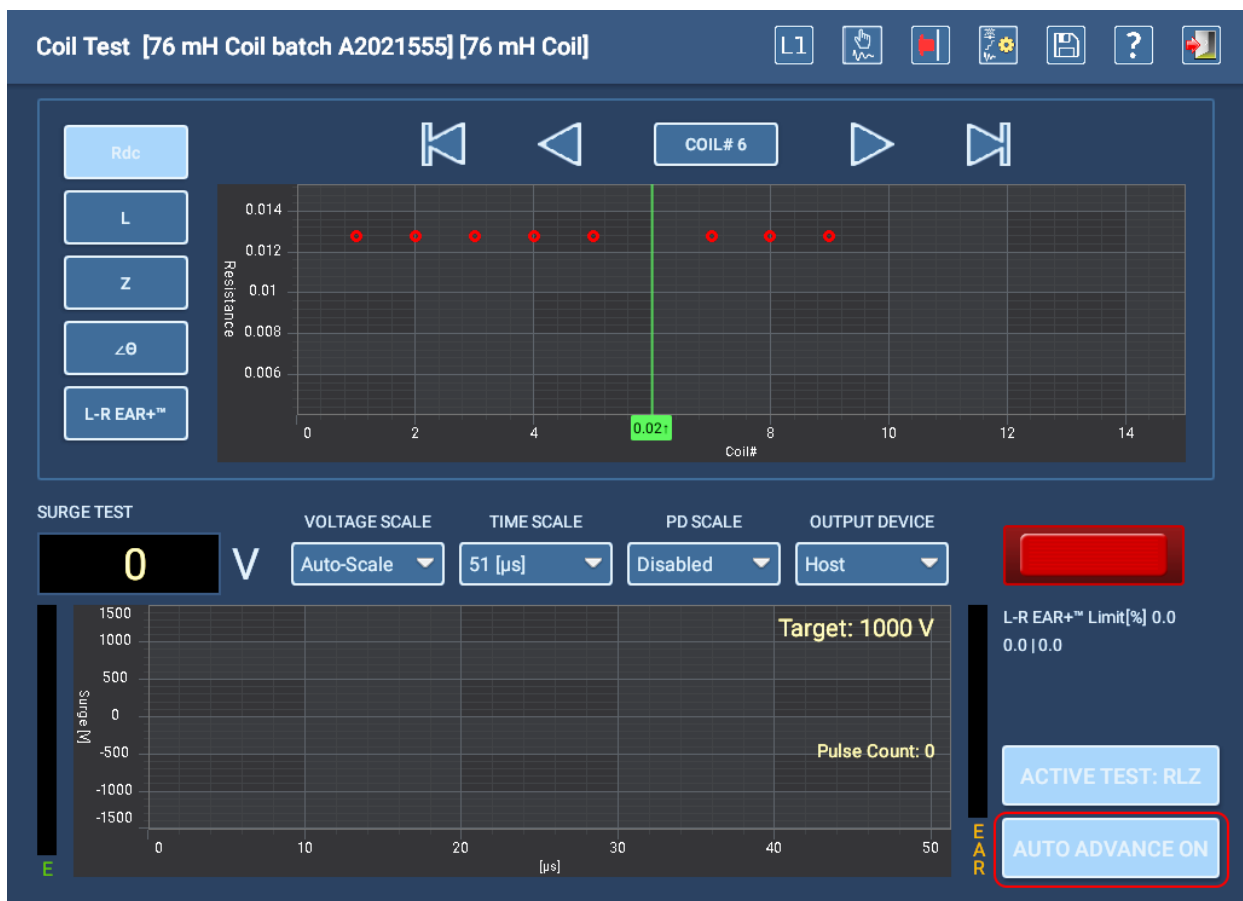
Fig 100: Coil Test screen with example RLZ test in progress.
