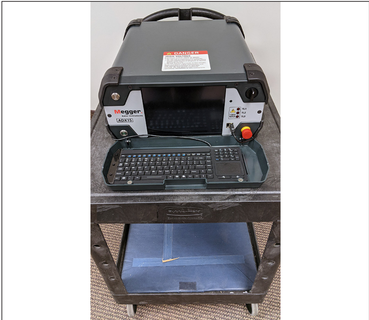
Fig 20: ADX resting on work cart; all bottom bumpers making full contact; wheels locked.
