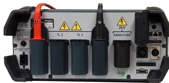
Fig 3: Inspect test lead receptacles and cables before each use.
