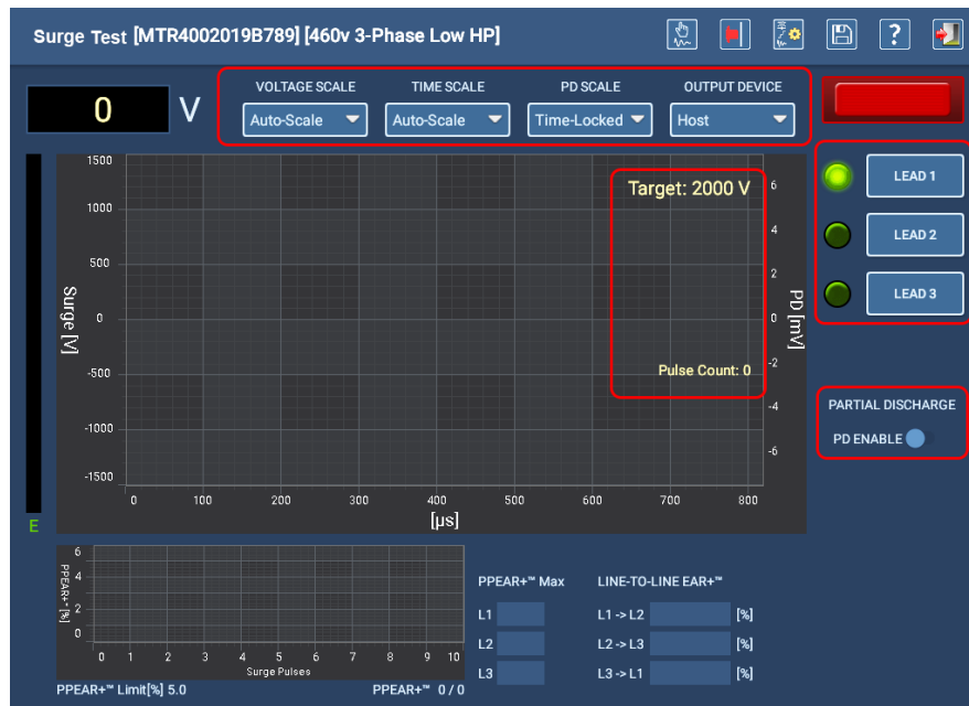
Fig 86: Manual Surge Test start screen; PD disabled.
