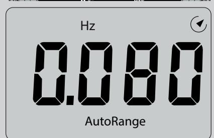
9. Press the Hz% button until "%" is indicate to read the % duty cycle in the display
