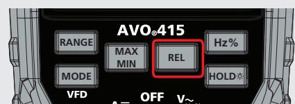
**NOTE :** The Relative function does not operate in the Frequency function.
