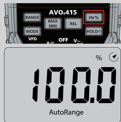
13. Press the Hz% button to return to current measurement
