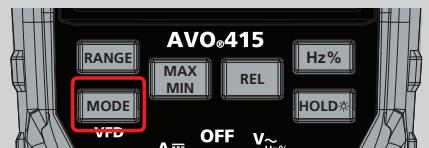
3. Turn the meter on while holding the MODE button
