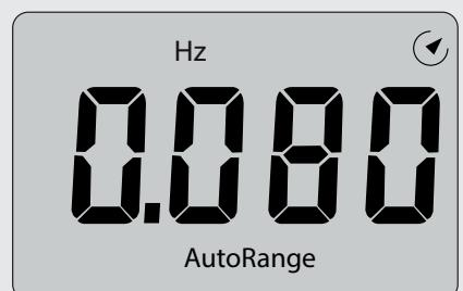
11. Press the Hz% button until "%" is indicate to read the % duty cycle in the display
