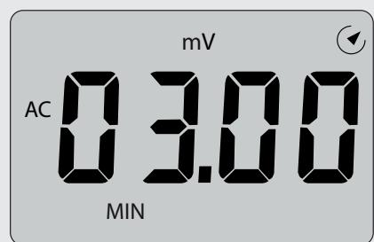
4. Press the MAX/MIN key again to activate the MAX/MIN recording mode. The display icon "MAX-MIN" will appear. The meter will display and hold the difference between the MAX and MIN reading
