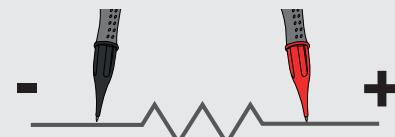
6. Touch the red test probe tip to the positive side of the circuit
