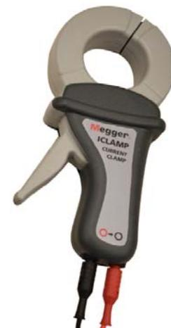
The mini active CT for the MGFL100 uses a flux gate technology, allowing a gap in the core. This also greatly reduces magnetization effects.
