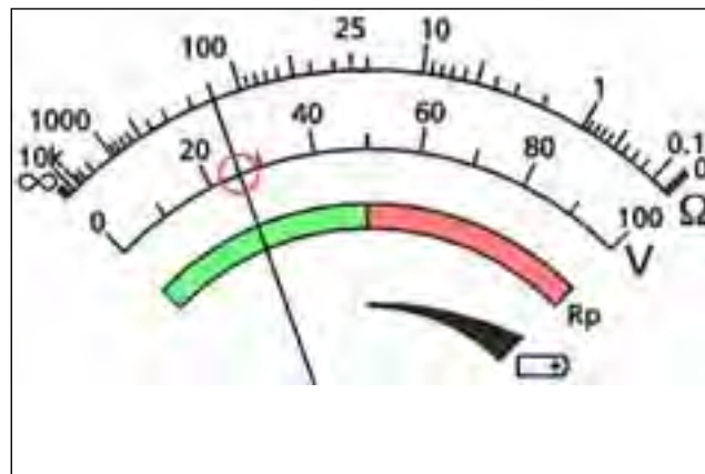
Figure 12: example ground noise voltage reading
