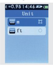
Press the **MENU** button to enter the setup menu. Use the **UP / DOWN** navigation buttons to highlight the DIST option. Press the **Enter** button.
