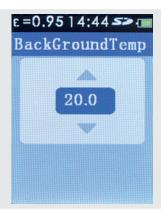
The BGT setting allows the user to set the background temperature.
