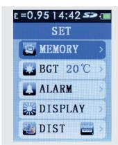
If required, the ALARM setting allows user to preset either or both a high and low threshold temperature alarm. A tone will sound when the high / low thresholds are viewed.
