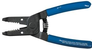
This truly metric wire stripper/cutters cuts, strips, loops, bends, and gauges stranded wire. Comfortable, plastic-covered handles reduce fatigue. Serrated nose jaws to bend, shape or pull wire; holes for looping wire ends.
