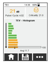
The bar at the bottom shows the maximum value measured within the last 10 measurements. The average measurement displayed (Avg) also refers to the last 10 seconds.
