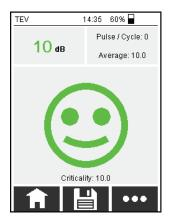
The average measurement shown is calculated from the level values measured for the last 10 seconds.
