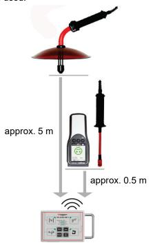
When performing acoustic measurements with the demonstrator box, the frequency has to be set to 40 kHz (see page 50)!
