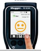
The current measurement screen is saved as a screenshot. A keypad for entering the file name appears. Pressing the button saves the screenshot in the data folder for the current measurement. The software then immediately returns to the measurement screen.
