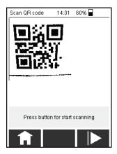
3. Hold the PD Scan up to the QR code and press the button. The integrated camera will now try to read the QR code, and will show its character string at the bottom of the display as soon as it was able to be scanned.
