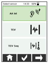
Pressing the required field on the touch display, or navigating to the required field using , followed by , allows the required operating mode to be started.
