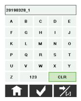
Briefly pressing the button allows the user to scroll through the list of fields on the touch screen. Pressing the button deletes the last character that was entered. Pressing and holding the button deletes all characters. You can switch to the numeric keypad by pressing 123. In addition to number keys, the keypad also has six freely assignable keys for frequently used text modules.
