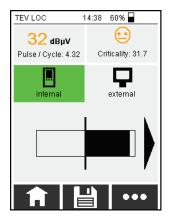
The black bar deflects in the direction of the sensor that is closer to the weak point. In the example, the weak point is considerably closer to the external sensor.
