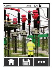
If the green cross indicating which can be enabled /disabled (see page 50) appears in the centre of the screen, it should be positioned as precisely as possible on the identified problem area or any other point relevant to the measurement when capturing the image. The green mark will then also be visible in the image file afterwards.
