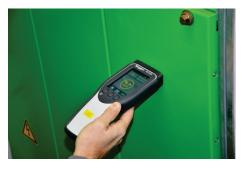
Flexible This external, acoustic sensor is specially designed for openings, air holes and gaps, airborne acoustic out of which the acoustic waves of the partial discharges can escape from the sensor switchgear.
