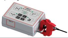
The front end of the PD Scan must be held against the contact surface marked with TEV 1 in TEV mode in order to be able to measure the pulses generated.
