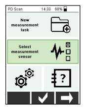
Pressing the **Select measurement sensor** field on the touch display or pressing opens the menu for selection of the operating mode.
