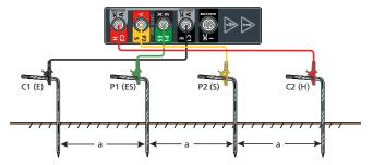
The Wenner method is the most common with the pins / stakes equally spaced in a line. The resistivity is calculated in the equation:
