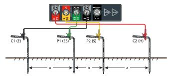
The Schlumberger method has the potential pins / stakes closer together, with a<2b. The resistivity is calculated in the equation:
