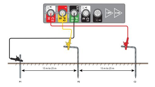
**Important:** The current stake / pin, potential spike and earth / ground electrode must be placed in a straight line.
