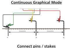
**Note:** Set up test leads and stakes as required by each test (do not connect the test leads to the instrument):
