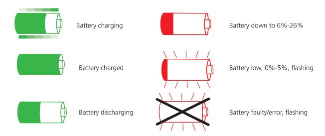
When running from the battery, the above will indicate the current state of charge (the icon will be filled proportionally to the state of charge). When the battery is charging, it will show an animation that starts with the current state of charge and fills the indicator to 100 %, then repeats. Once the battery is full, the animation will stop. If the charger is connected (and on), but unable to charge the battery, the icon will flash. Capacity and typical charge life 10 hours max.
