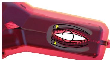
Megger clip being tested with IEC standard test finger for creepage and clearance.
