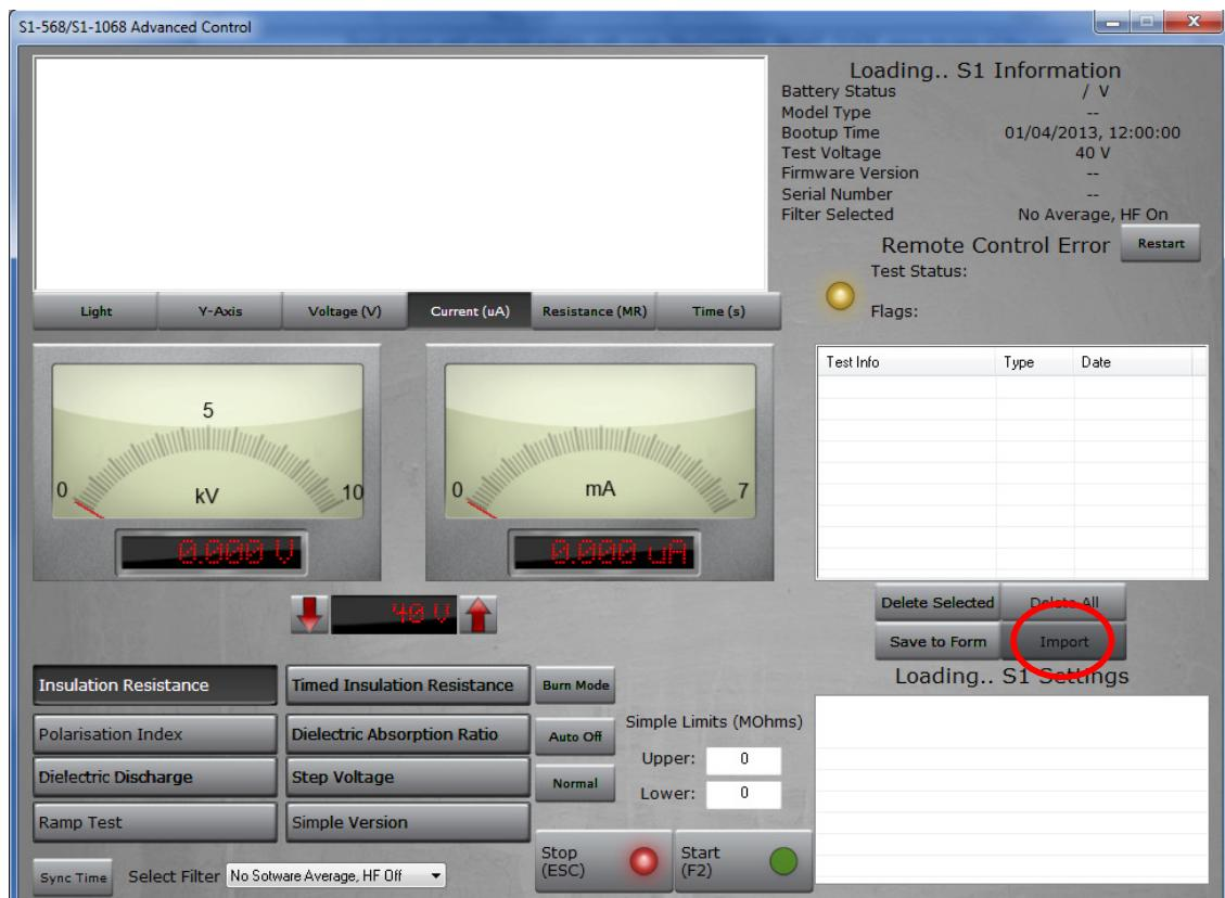
To activate the Import/Live Stream Control application click the **Import** soft button (circled) in the remote control application.
