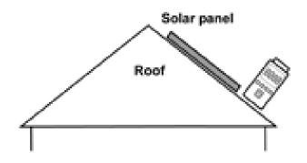
For a more accurate measurement at the optimum angle or position, the universal camera mount on the rear of the meter may be utilised. For easy reading the measurement on the meter can be retained on the display by pressing the HOLD button.
