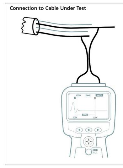
Connect the test lead to the cable under test. Connection may be made to a live power system with a voltage to earth (ground) less than 150 V with an installation (over voltage) category of I V or lower.
