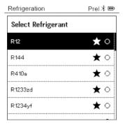
Setting the refrigerant: Press [▲] or [V] to select the refrigerant and press [Menu/Enter] to confirm.
