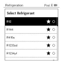
Setting the refrigerant: Press [▲] or [▼] to select the refrigerant and press [Menu/Enter] to confirm.
