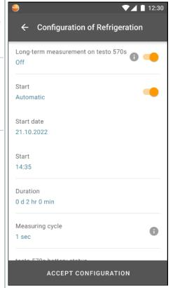
If the long-term measurement option is enabled, the configuration menu shows the remaining battery and rechargeable battery capacity and the maximum possible duration of the long-term measurement.
