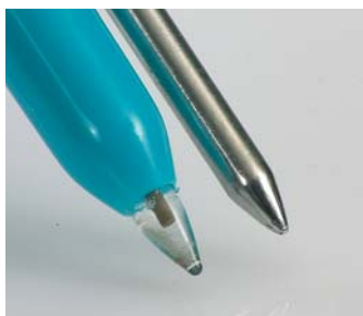
pH2 probe head for semisolid substances
