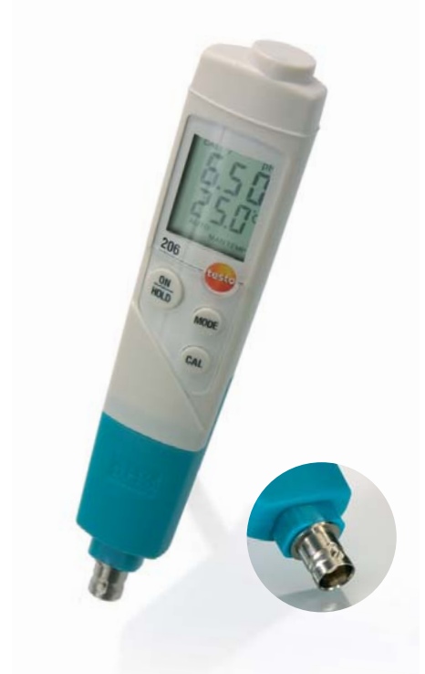
pH3 probe head with BNC interface
