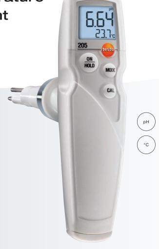
The testo 205 is a robust food penetration measuring instrument for temperature and pH values, with automatic temperature compensation. The robust penetration measurement tip is exchangeable and insensitive to dirt thanks to the hole diaphragm.
