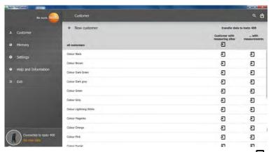
In order to have the relevant customer data available in the instrument for measurements on site and to assign new measurements on site to measuring sites, all customer data and measuring site information is transferred to these customers by clicking the left 2.
