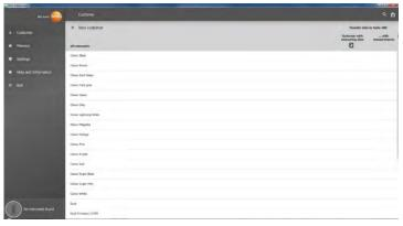
As long as the testo 400 is not connected to the computer, No Instrument found is displayed at bottom left.
