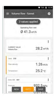
6 Apply: the current reading is applied.
