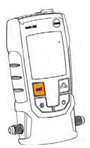
Adjusting the alarm threshold causes an alarm to be triggered when the set value is exceeded.
